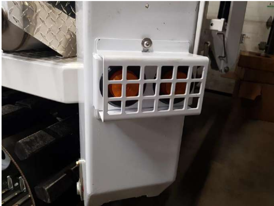
Front Outriggers: Amber Clearance & Turn Signal Lights
